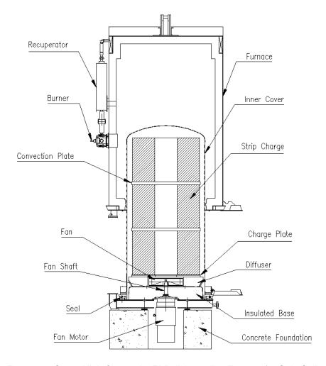
Figure 1. – Super-High Convection™ Bell Annealing Furnace for Strip Coils
