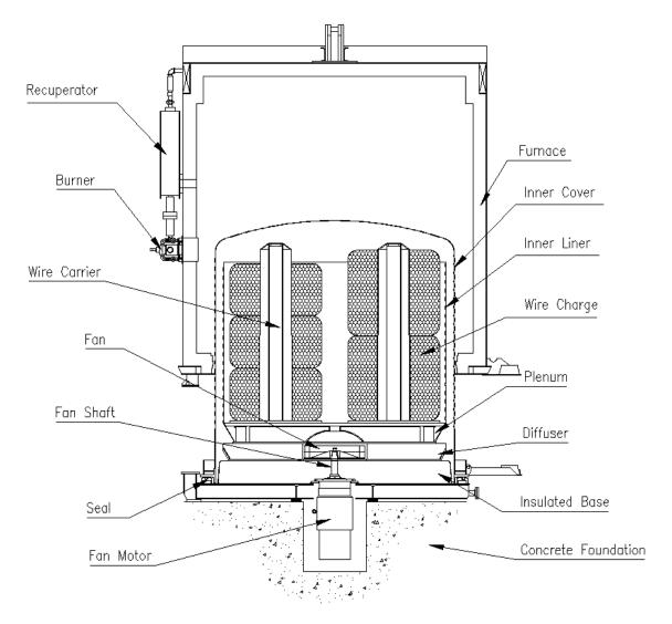
Figure 2. – Super-High Convection™ Bell Annealing Furnace for Wire Coils
