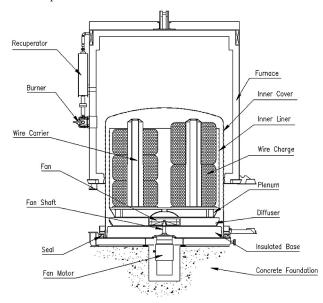
Fig. 1 — Bell-type batch annealing furnace.
