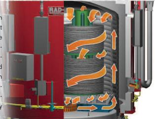
AC/APEx<sup>™</sup> The patented RAD-CON AC/APEx™ system adds another level of process optimization. Combining gas stream analysis with closedloop process control results in a clean, decarb-free charge every cycle.
